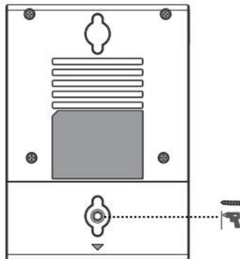
2. Wall mounting can be achieved by hanging the equipment on a screw suitable for the size and distance of the two holes above and below the back shell.
